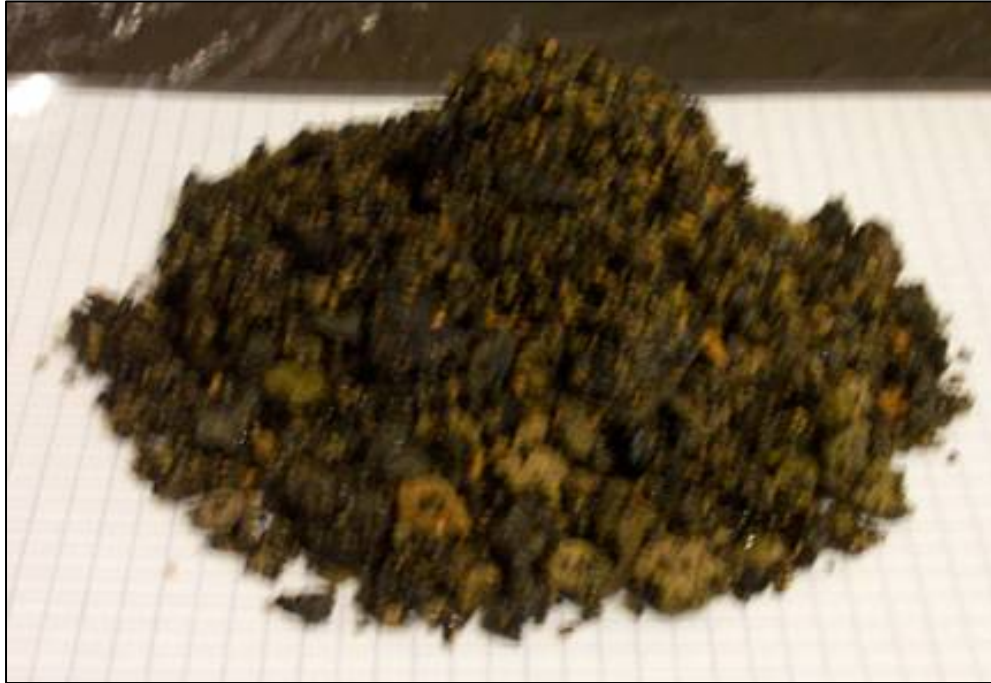
—— Bottom Ash Sample Collected on a Cofire Day (not necessarily a typical sample for a cofire day)
