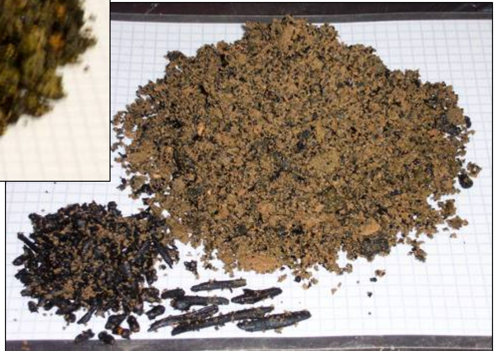
Same Bottom Ash Sample, with Unburned Biomass Separated ——
