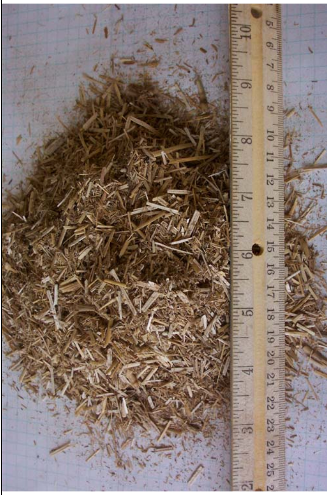
2" screen, 13 tph out of eliminator
