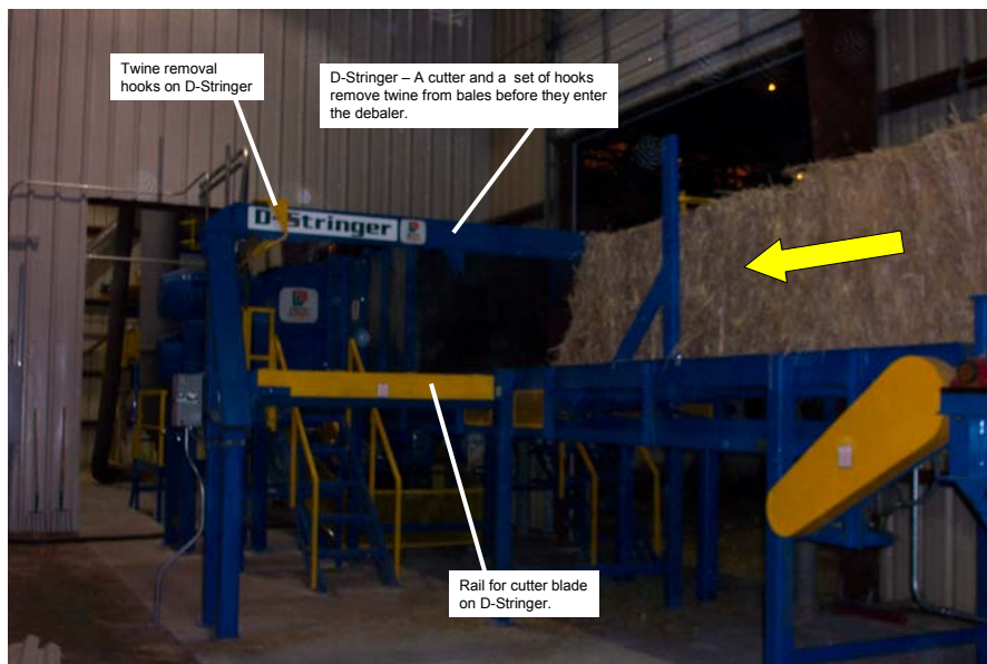
Bales on bale conveyor approaching D-Stringer and Debaler.
