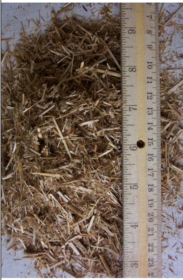
6" screen, 11 tph out of eliminator
