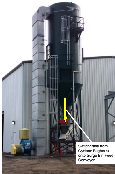
Cyclone Baghouse that conveys ground switchgrass from the "Eliminator" onto the Surge Bin Feed Conveyor and removes and filters dust from the processing area.
