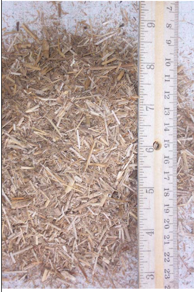
1" screen, 13 tph out of eliminator
