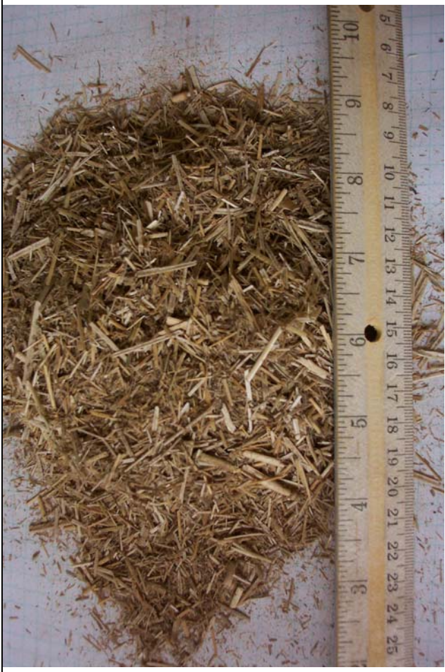
3" screen, 12 tph out of eliminator
