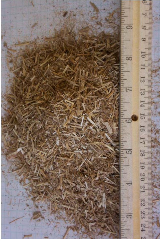
1/2" screen, 12 tph, out of eliminator
